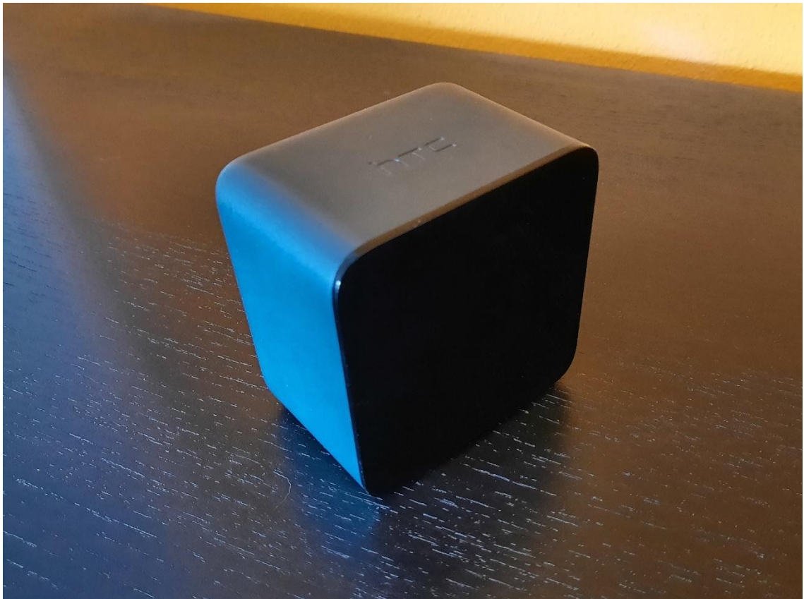
FIGURE 3: ONE OF THE BASE STATIONS THAT ARE USED FOR TRACKING THE HTC VIVE AND ITS CONTROLLERS.
